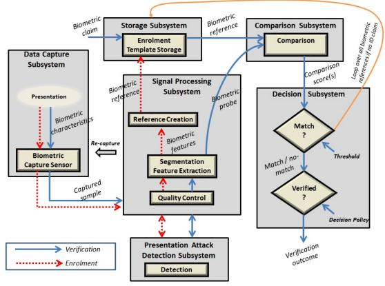
Figure 1. Generic representation of a TOE
